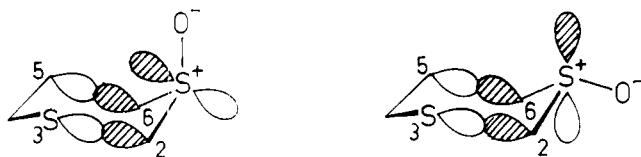
Figure 1. Proposed interaction of sulfoxide 3p orbital with \sigma^* orbitals of C(5)-C(6) and C(2)-S(3) fragments is better when the lone pair is equatorial and the oxygen is axial.
